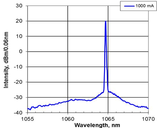
\* Performance is given for the 1064nm device. Similar performance is expected for the other wavelengths in the 1010-1090nm range.
